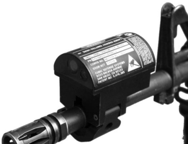
MILES 2000 Transmitter positioned on an M16A2 Rifle. (Consult your local TASC for detailed mounting instructions and supporting offset target data)
