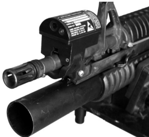
MILES 2000 Transmitter positioned on an M4 Carbine, with M203 attached. (Consult your local TASC for detailed mounting instructions and supporting offset target data)
