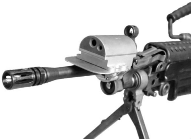
MILES 2000 Transmitter positioned on an M249 SAW/LMG. (Consult your local TASC for detailed mounting instructions and supporting offset target data)
