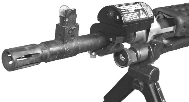
MILES 2000 Transmitter positioned on an M240B Medium Machine Gun. (Consult your local TASC for detailed mounting instructions and supporting offset target data)
