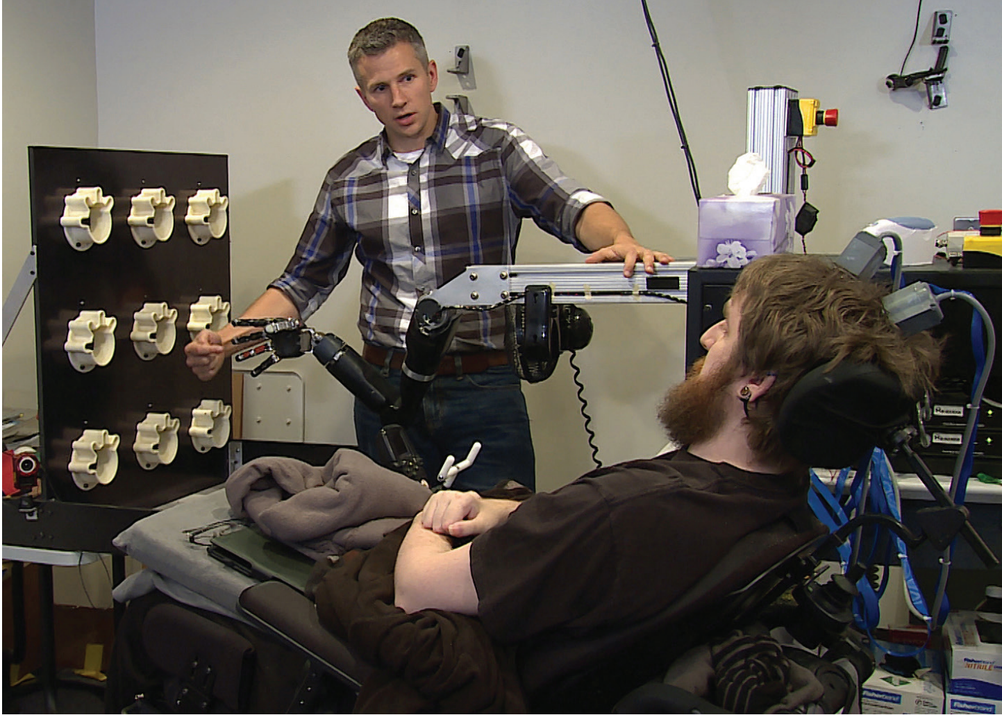
Nathan, a participant in DARPA's Revolutionizing Prosthetics program, controls a robotic arm with his brain and feels what the limb touches.
