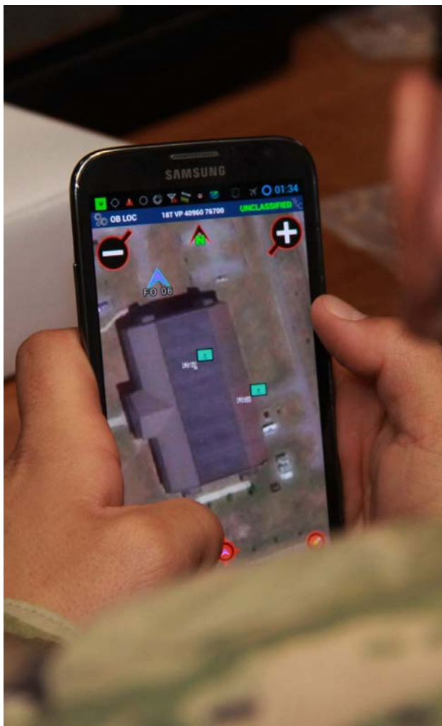
A soldier with 3-6 FA, 1BCT, 10th Mountain Division, navigates the new Precision Fires-Dismounted system that allows soldiers to view live-streaming full-motion video from unmanned aerial vehicles through an app on approved smartphones. The ubiquitous cellphone technology used worldwide owes its existence in part to the development of the GaAs semiconductor industry made possible by DARPA-funded research.
