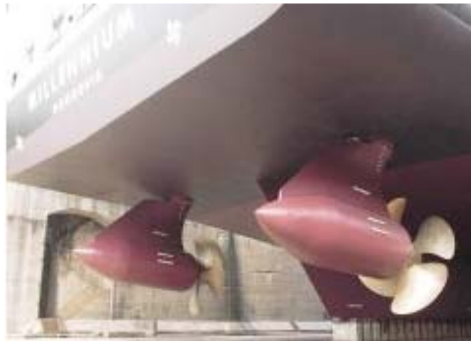
Figure II-4. POD Propulsion Used on Commercial Shipping (From: Rolls-Royce).
