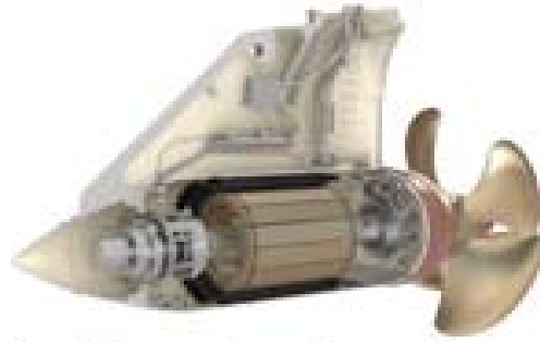
Figure II-5. Pod Propulsor Called Mermaid (From: Rolls-Royce).
