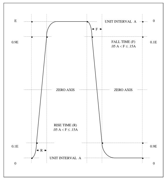
Rise and Fall Times (0.1 to 0.9 of the peak-to-peak voltage, E) shall be approximately equal and shall exceed 5% but shall not exceed 15% of the unit interval, A, at either 1200 or 600 bits per second
