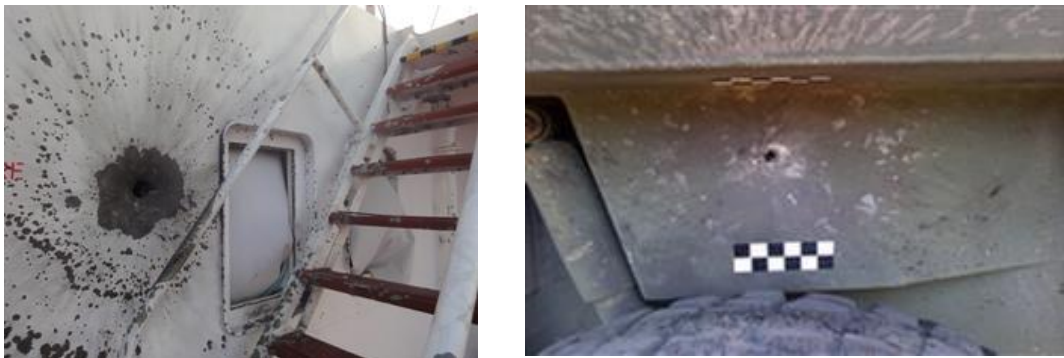
Figure 2: Comparison of a suspected RPG strike (LHS) to a controlled RPG strike (RHS)
