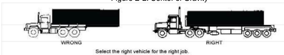
Figure E-3. Selecting a Vehicle for the Load
