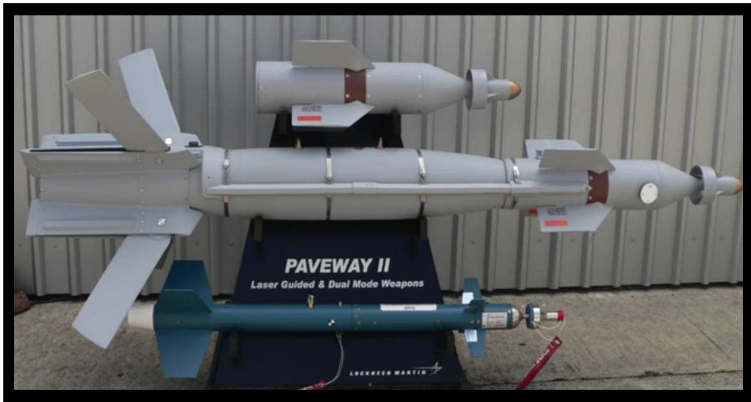
“Paveway” guidance systems “convert thousands of dumb bombs into smart bombs.” Paveway kits attach to a variety of warheads, and consist of a semi-active laser (SAL) seeker, a computer control group (CCG) containing guidance and control electronics, thermal battery, and pneumatic control augmentation system (CAS).
