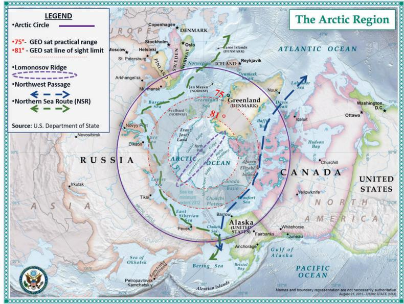
**Figure 1: The Arctic Region.** The smaller red circle (81°3') is the maximum latitude beyond which a geostationary satellite (GEO) is unable to provide coverage because it is below the local horizon. Operationally, a GEO satellite's limits are several degrees lower due to receiver noise from atmospheric refraction, frequency interference due to Earth's thermal emission, line-of-sight obstructions, and signal reflections with ground structures at approximately 75°.<sup>4</sup>
