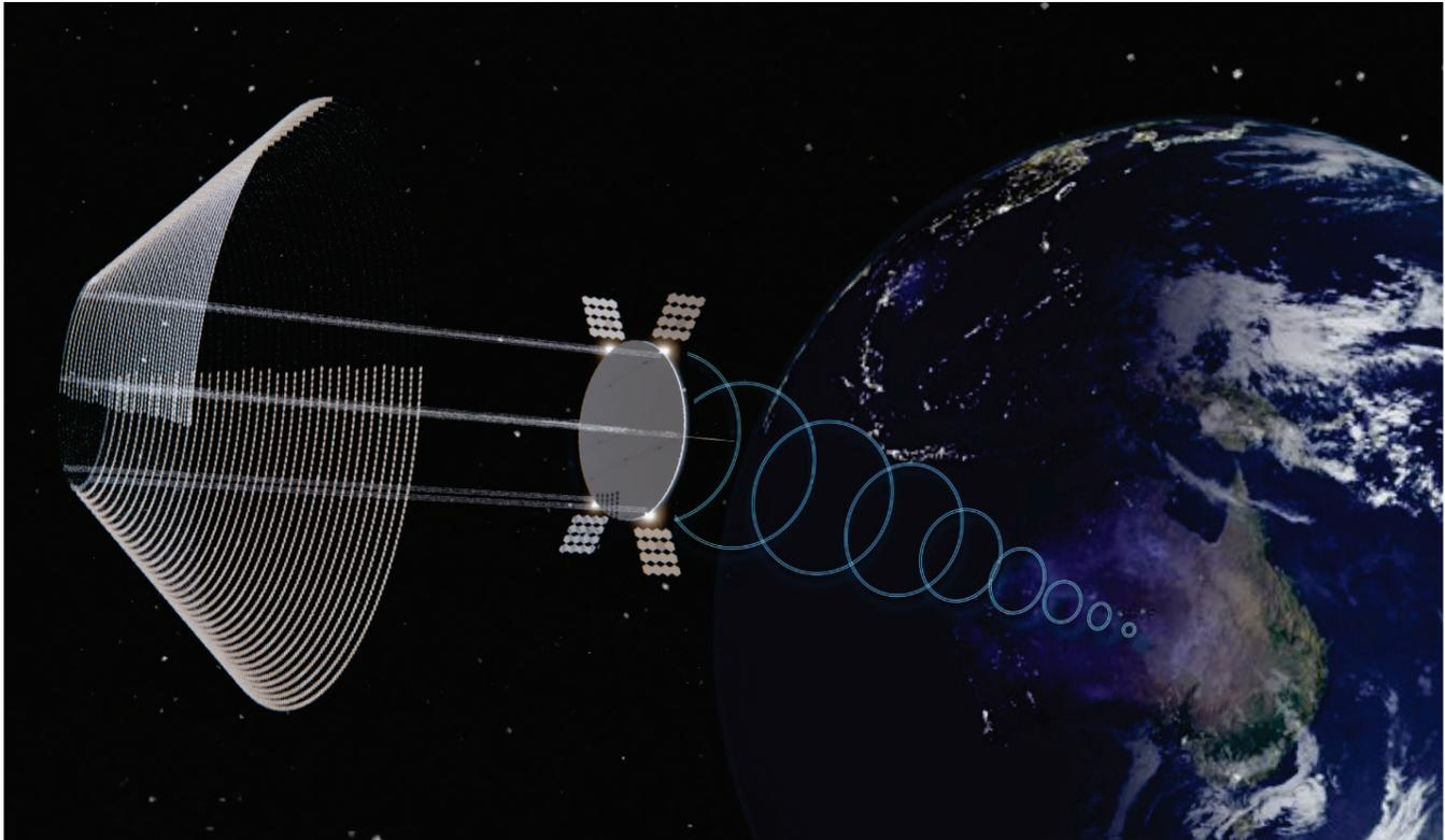
**Figure 3: Highly modular SPS-ALPHA Mk-III space solar power system concept with light-weight structure and heliostat reflector array, transmitting power to Australia. (Image courtesy of John C. Mankins)**
