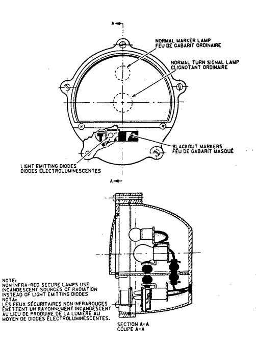
FIGURE 2 - INFRA-RED BLACKOUT COMPOSITE LAMP FRONT, TURN, PARK AND MARKER / FEU MASQUÉ
