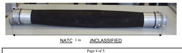
T-25TEST METHODEdition no. 1 dated 15/09/2000HYDROSTATIC TESTS: ELONGATION AND TWISTING OF HOSES AND HOSE ASSEMBLIES
