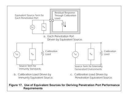
(3) Penetration Equivalent Source. The equivalent source term for each conducted EME for each penetration port is then applied to the same calibration load used to derive the residual response (Figure 17c). The response through the calibration load is the conducted EME response. A Fourier transform of the transient conducted EME (time domain) is required to provide the response as a function of frequency. The narrowband EME response can be used directly.
