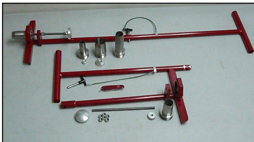
Figure A3.2. - An example of a sampling tool for obtaining uniform soil increments (CRREL).
