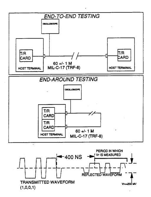
Figure 10 Composite Noise Test Set-Up (Figure 11 of 4153)
