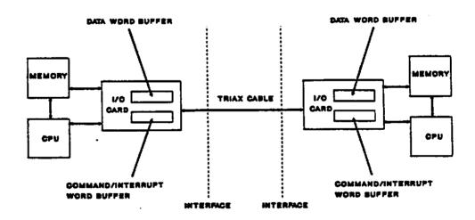
Figure 2 Typical Interface Architecture
