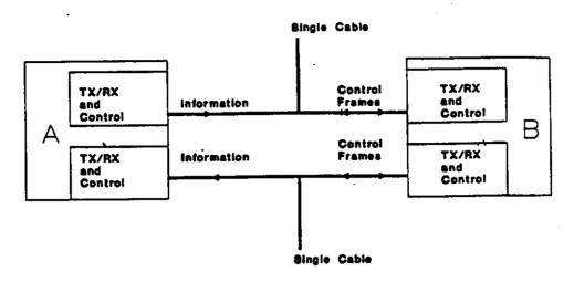
Note that A or B is either a Source or Sink depending upon which cable is being considered.
