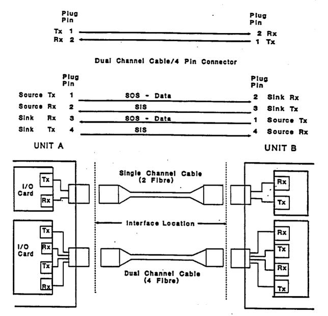
Figure 12 Channel Implementation and Location of Interfaces
