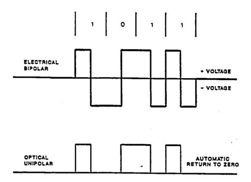
Figure 13 Interface Waveforms
