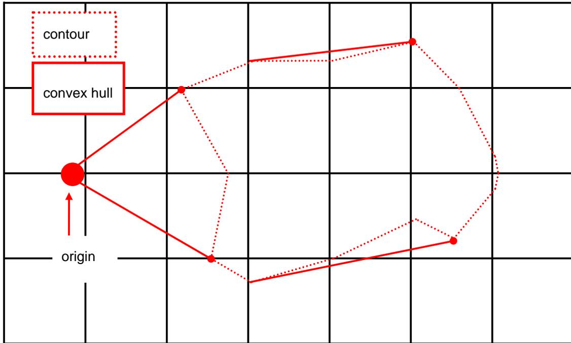
Figure 7.1 — A convex hull corresponding to a contour in two dimensions
