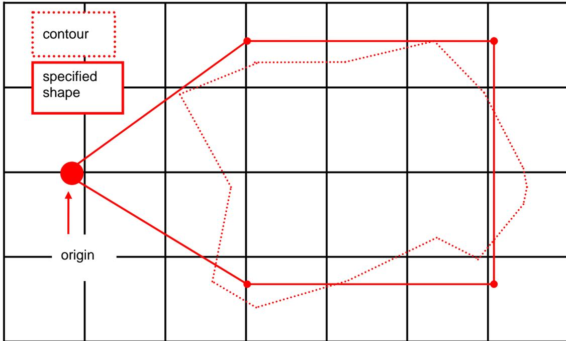
Figure 7.3 — A specified shape partially covering a contour in two dimensions i.e. the contour crosses the boundary of the shape and is not fully enclosed within the shape.
