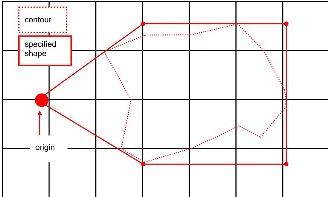
Figure 7.2 — A specified shape covering a contour in two dimensions i.e. the contour is fully enclosed within the shape.
