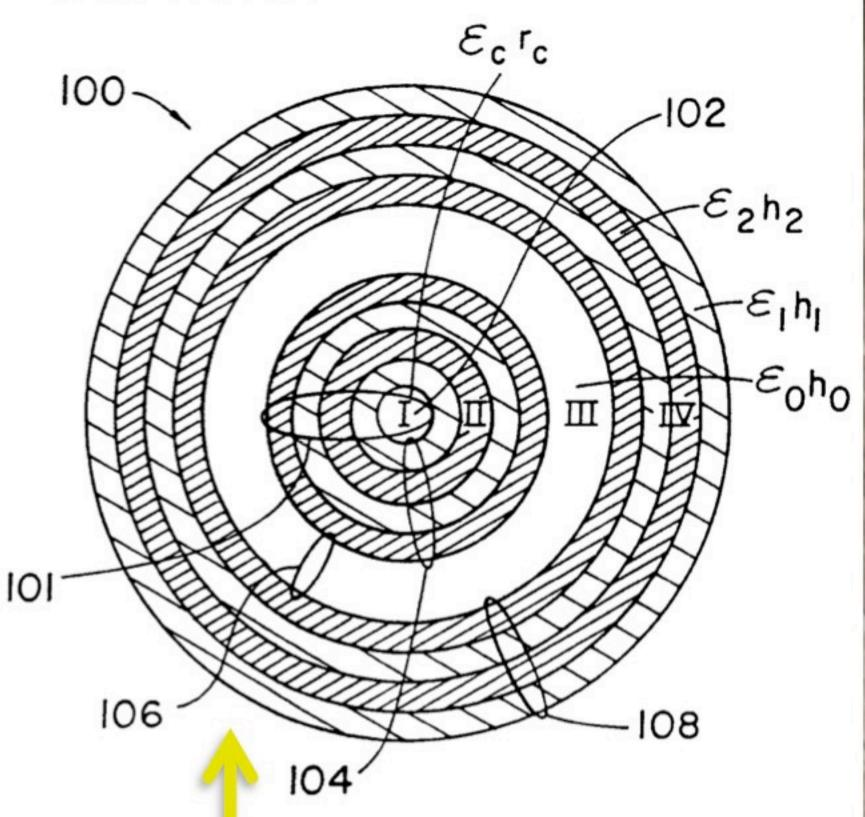
Example of concentric ring resonator waveguide (Fig. 1 from patent US 6573813 B1)
