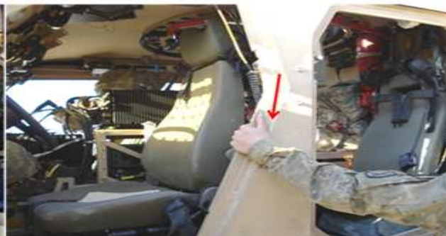
Fig 2: Improper Hand Hold
