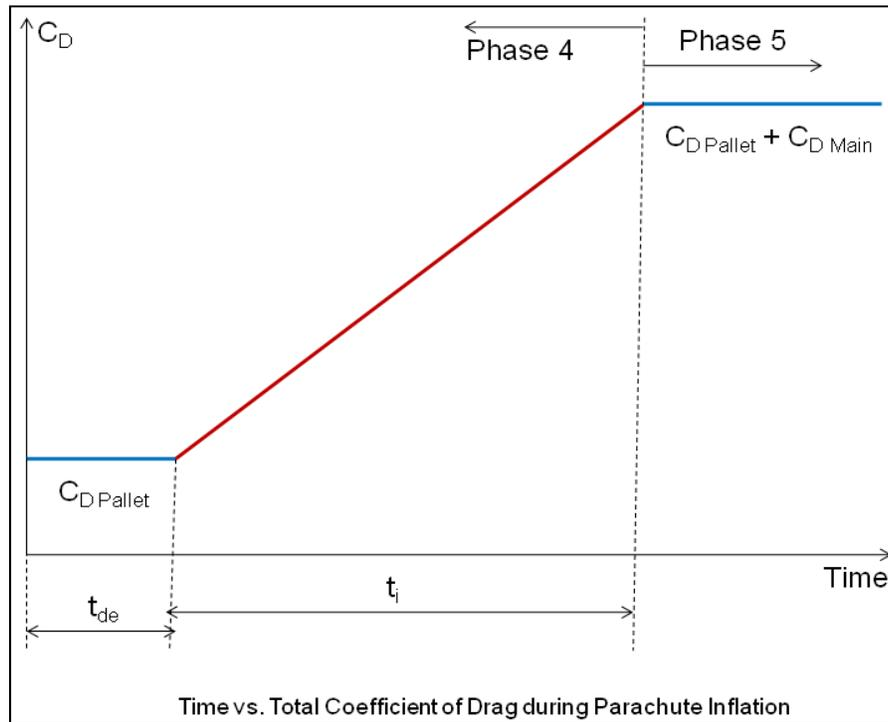
**Figure 5. Time vs. Total Coefficient of Drag during Parachute Inflation**
