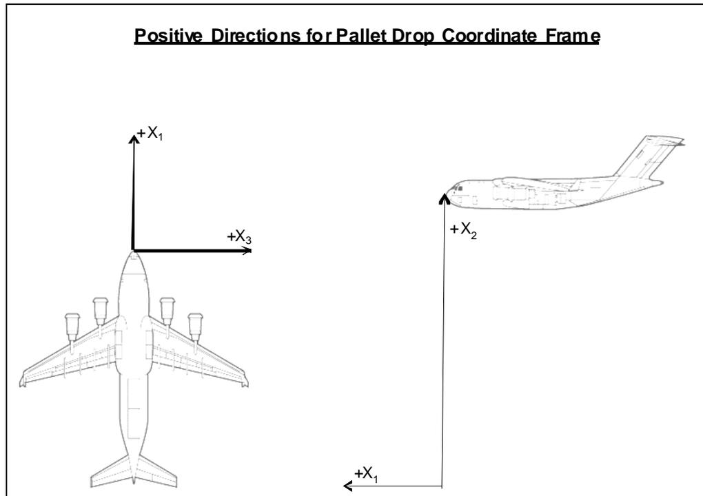
**Figure 1. Positive Directions for Pallet Drop Coordinate Frames**
