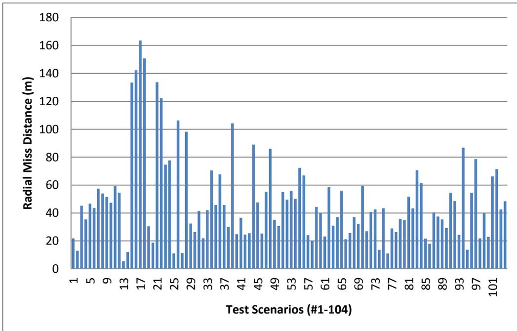
**Figure 11. Radial Miss Distance between JPADS and Prototype Produced CARPs**
